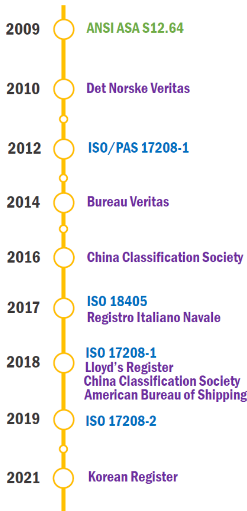
Figure 1: Timeline of URN measurement procedures. National standards (green), international standards (blue) and classification societies’ notations (purple). Just first issues of the documents are gathered. Consulted documents for this report are available in Table 3.
